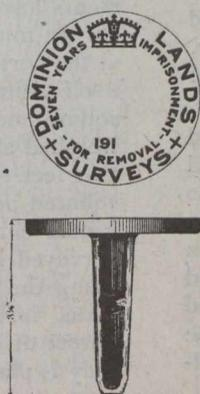
Fig. 2. Short Survey Post for planting in rock.
