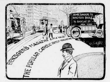
AN INGENIOUS DEVICE FOR PRINTING ADVERTISEMENTS ON ASPHALT PAVE-MENTS BY MEANS OF AN AUTOMOBILE.
