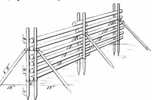
The cost for new material is very small, as old stakes that are too short for cross stakes for worm fence can be used, or a cedar or oak rail will make two stakes or a stake and a brace; the wire will cost about one cent per rod. I think two men could prepare stakes and braces and put up 20 rods y. In this fence there are no wide spaces
