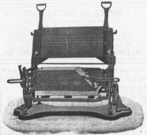
This Machine makes all blocks face down-"the only practical way "-allowing of a richer and finer facing, producing blocks that are perfect in appearance and impervious to moisture.
