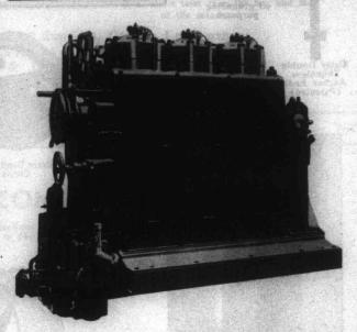
3 cyl. Gz single acting 2 cycle 100-125 HP. per cylinder With patent loop scavenge and oil cooled
