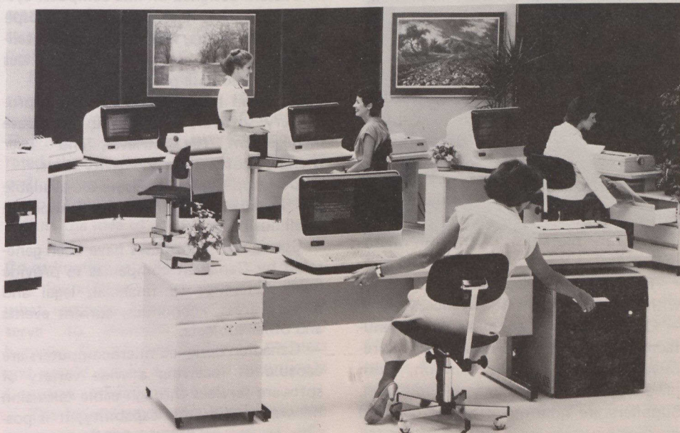
A version of the AES C20 made up of four work-stations connected to a central unit containing a microprocessor. Each of the four units can type up to 540 words a minute making the total output of the system 8 000 words a minute.
