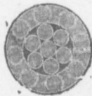
Locked Coil Aerial Cable or Colliery Guide.
