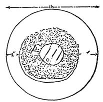
Fracture of Railway-Axle.
