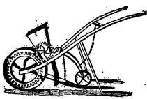
Having noted the increasing attention given of late years to the growth of roots, it has been my study to produce a drill which would be generally adapted to the sowing of every description of seeds. I finally decided on the one, of which the annexed cut is a representation, as the most universally applicable.
