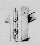
and down at will. The lower end is pointed and the upper end squared so that it may be readily turned with a wrench. The rod is fastened firmly to the side of the leg (one on each of the front legs), and turned down so that the point will dig into the floor just enough to hold it firmly.
