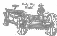
THE John Deere Spreader is a low-down spreader in which the advantage of big drive wheels is not sacrificed for the low-
