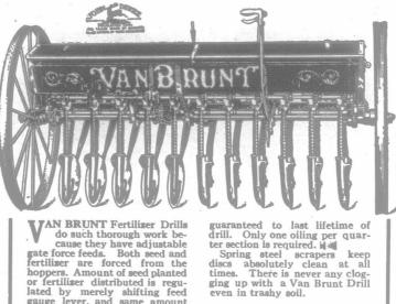
VAN BRUNT Fertilizer Drills do such thorough work be-cause they have adjustable cause they have adjustable gate force feeds. Both seed and fertilizer are forced from the hoppers. Amount of seed planted or fertilizer distributed is regulated by merely shifting feed gauge lever, and same amount passes through each tube into the ground. Each wheel drives half the teeds.
