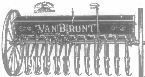
**V**AN BRUNT Fertilizer Drills do such thorough work because they have adjustable gate force feeds. Both seed and fertilizer are forced from the hoppers. Amount of seed planted or fertilizer distributed is regulated by merely shifting feed gauge lever, and same amount passes through each tube into the ground. Each wheel drives half the feeds.
