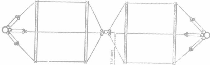
"BT" Slings are made of the best Manilla rope, and will trip no matter how they are placed on the wagon or how the bundle may twist.
