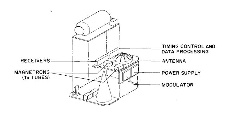
FIGURE 7-7: EXPLODED VIEW OF KU-BAND RADAR ACCOMMODATION
