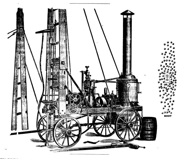
(HIS DRILL does the work without the use of Diamonds, using as a substitute Chilled Steel Globules, or as they are commonly called, shot. These are inexpensive, costing in actual work about ten cents per day; whereas, diamonds are very expensive, a single one often costing from \$80 to \$100, thus showing the difference in cost in case of loss of tools. It is THE BEST, CHEAPEST, and MOST EFFECTIVE CORE DRILL made for Prospecting Quarries, Coal Lands, Sinking Wells and the like.
