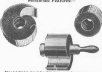
The Link-Blades closed for skimming, open for cleaning and held by standard for convenience in cleaning.
