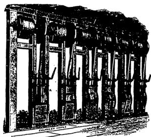
When two or more knives are run with one belt, all must stop when the belt is stopped to set bits or from any other cause. Our Machine has a belt for each knife, hence but one knife stops at a time. This great advantage should not be overlooked by purchasers. Time is money. Our Machine cuts more excelsior in a given time than any other machine. Get our circulars and prices.
