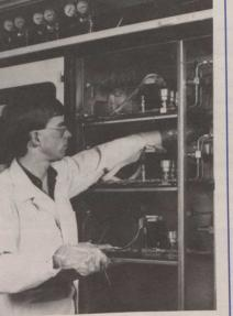
Process Technology Limited employee examines gas panels in a low-pressure chemical vapour deposition system.
