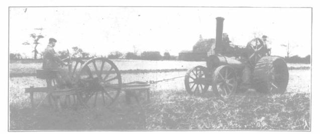
CULTIVATING WITH TRACTION ENGINE TO BREAK UP A HARD PAN.
