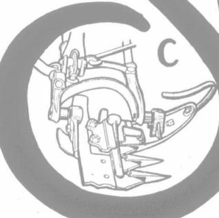
Illustration C shows you the Large Bearings used in our "stay-tight" connection between Cutter Bar and Main Frame of Mower. Unlike Small Pins used on other mowers, they do not wear down hurriedly and permit connection to work loose. Instead, they fit precisely together and have no chance to wear. That's why it is called the "stay-tight" connection. That's why there is no time lost on the field—no blacksmiths' bills to pay.
