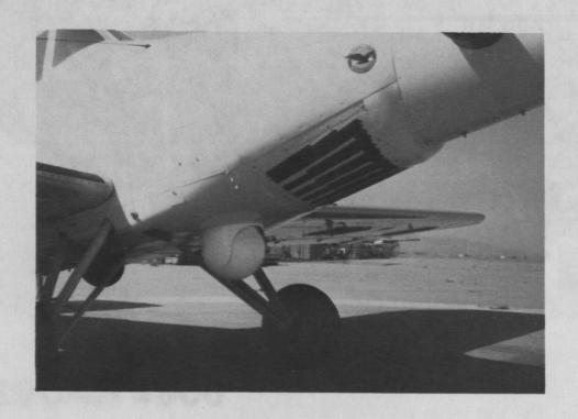
Figure 11. Two Honeywell Gimbaled Mark III FLIR systems mounted fore and aft under the fuselage of an Ayres S2/R Turbo Thrush aircraft. (Courtesy of Dave Dorschner, Aviation Resource Management.)
