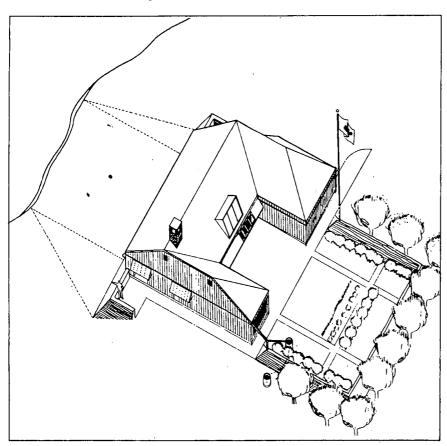
The design of this house accommodates many energy-conserving devices. Domestic hot water is heated by three solar collector panels. The 3500 sq. ft. of space is heated by wood and oil forced warm air furnace. Vestibules and insulated doors prevent loss of warm air and infiltration of cold and the windows have insulating glass and insulating storms, as well as insulated curtains hung from a no-draft valance.
