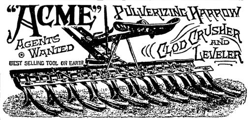
Subjects the soil to the action of a Steel Crusher and Leveller, and to the Cutting, Lifting, Turning Frocess of Double Gangs of Cast Steel Coulters. Immense cutting power. ing, Levelling and Pulverizing performed at the same time. Entire absence of Spikes or Spring Teeth avoids pulling up rubbish. Only Harrow that cuts over the entire surface of the ground.
