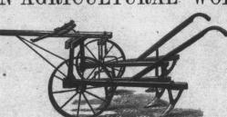
Two-horse straddle-row Corn Cultivator, adjustable for width and depth, the best machines made for surface cultivation, costs little more than the one-horse machine.
