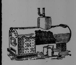
This is composed of 90% Asbestos fibre and a cementing compound forming a light, porous covering, partaking of the nature of a felt and a cement, to be applied with a trowel to Steam Pipes, Boilers, etc., while heated. This is recommended for all steam heated surfaces. Furnished dry, to be mixed with water to the consistency of mortar, and can easily be applied by unskilled workmen.
