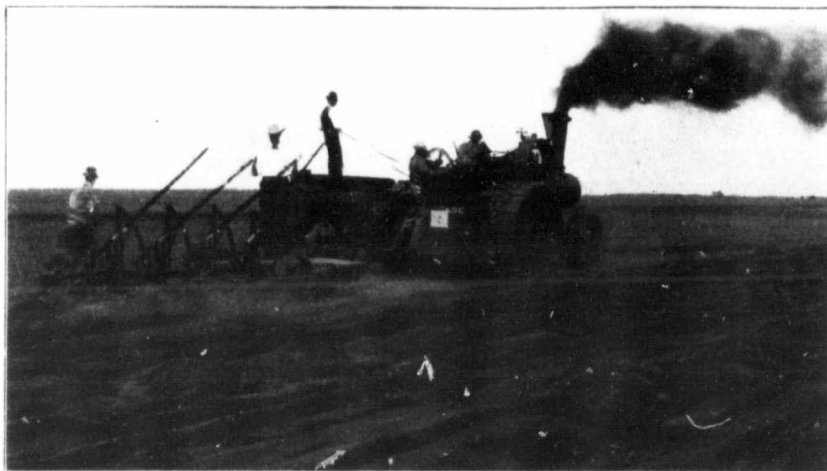
The Case 12 h.p. Steam Tractor pulling a 4 bottom Cockshutt Engine Gang
