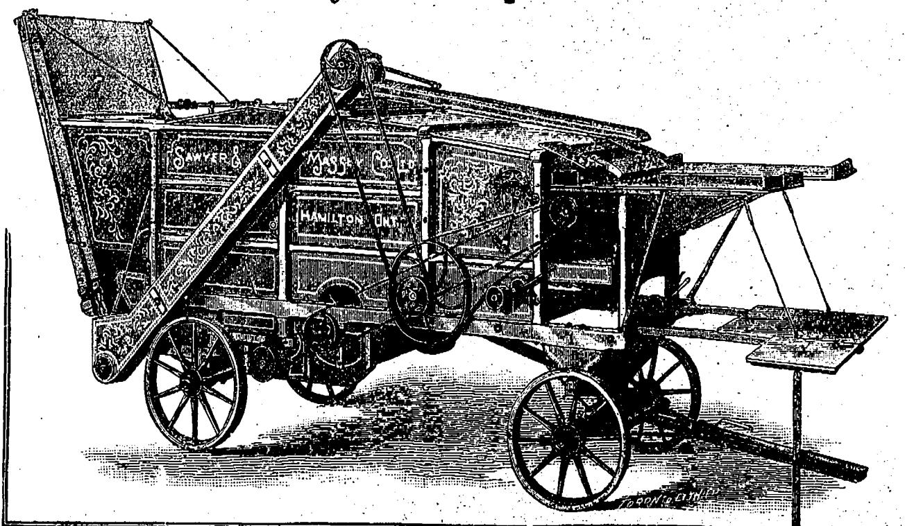
This is the Latest Improved Style, with Cast Iron Sides, and Cylinder Cap. Unsurpassed for Threshing Wet Grain, Peas, and all kinds of Grain and Seeds.
