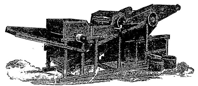
We manufacture our undershot thresher in four styles, 1st as shown in the cut; 2nd as in cut but with the addition of tailing elevator to carry tailings leach to the fee ling table. 3rd as in cut except that the grain fails into three coxes instead of measures and in this style we are able to separate the grains as is specially asked for in some parts of the Province. 4th We also manufacture the old style
