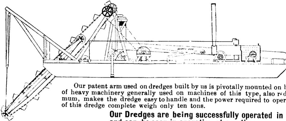
Our patent arm used on dredges built by us is pivotally mounted on boat and does away with a large amount of heavy machinery generally used on machines of this type, also reduces the cost of operation to a minimum, makes the dredge easy to handle and the power required to operate very small. The machinery parts of this dredge complete weigh only ten tons.
