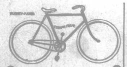
The cushion frame of the Massey-Harris is a good-road maker. It takes all the ruts out of the road. The jolting is absorbed in the air cushion of the frame.
