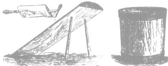
Fig. 1.—Fleshing knife. Fig. 2.—Fleshing beam. Fig. 3.—Tub for soaking skins.
