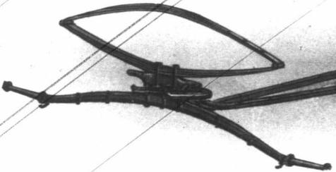
**Cut No. C**—High arch end spring gear. This will only be furnished as illustrated, unless specially ordered. (If furnished on any other job an extra charge will be made.) Furnished regularly with wood bars; Bailey loops when ordered. Height of wheels, 2 feet 11 inches and 3 feet 3 inches, with rubber tires, or 3 feet 1 inch and 3 feet 5 inches with steel tires.
