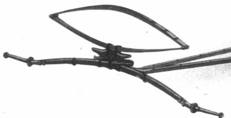
**Cut No. D**—High arch new style gear. Axles swedged top and bottom, and tapered, wood centres as illustrated. Can be furnished on any standard road wagon or buggy at an extra price. Supplied regularly with Bailey loops. Height of wheels, 2 feet 11 inches and 3 feet 3 inches with rubber tires, or 3 feet 1 inch and 3 feet 5 inches with steel tires.
