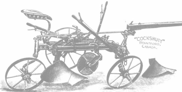
WHEN this plow is set for width and depth of furrow, it practically runs itself. All the operator has to do is to drive his horses. Your son can do that. By means of a special device the plow is locked when raised and locked down when
