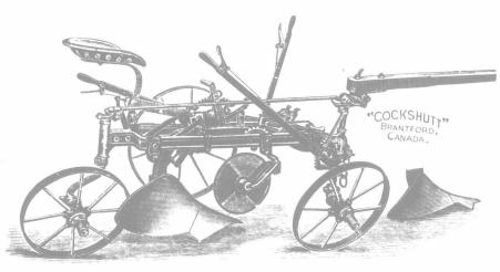
HEN this plow is set for width and depth of furrow, it practically runs itself. All the operator has to do is to drive his horses. Your son can do that. By means of a special device the plow is locked when raised and locked down when
