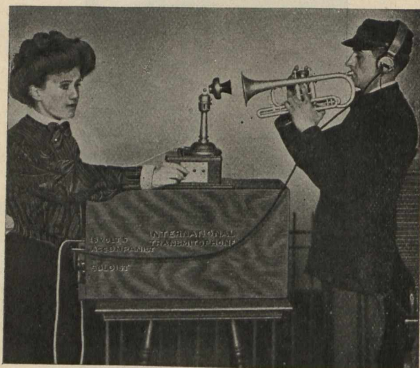
Fig. 3.—Sending Station Apparatus, with Cornetist Playing Directly in Front of Transmitter.
