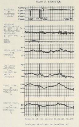
of turbulence, and local weather conditions. Completed tapes with the navigator's data logs and route maps are sent to NAE for analysis. Events with significant turbulence or large temperature changes along the flight path are selected for more detailed study, including an analysis of meteorological conditions by Graeme Morrissey, a research meteorologist with the Atmospheric Research Section, Meteorological Service of Canada.
