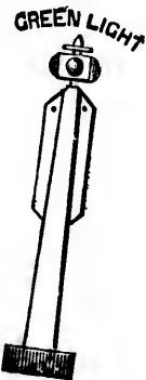
The *Caution* signal to slacken speed is shewn during daylight by the semaphore arm being raised to an angle (thus
