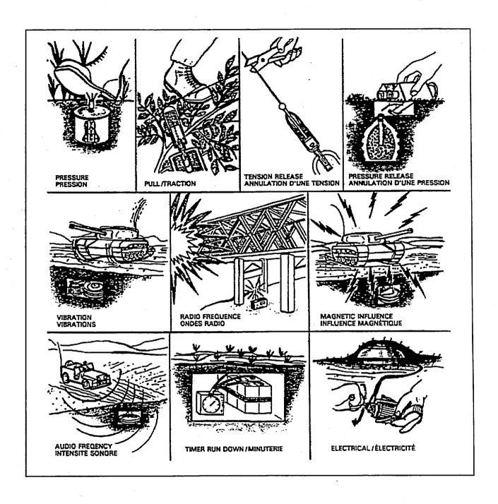
FIGURE 1 - DIFFERENT TYPES OF FUSE INITIATING ACTIONS FOR LANDMINES
