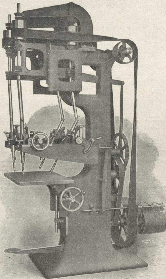
This Machine bores the four leg holes in 900 to 1,000 chair seats per hour. Tight and loose pulleys are 12 x 5 inches, and should run at 500 revolutions per minute. Floor space required for the machine is 4 x 6 feet. Weight of machine, 2,400 pounds.
