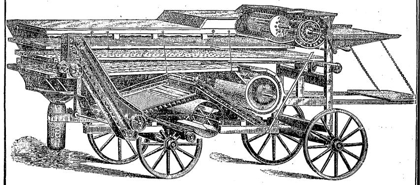
Skeleton Cut, showing Interior of the "Monitor" Clover Huller and Tailing Elevator.
