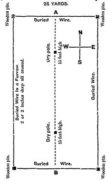
A B, Strong hooked pers to fasten the connecting wires that pass over the tops of the poles.
