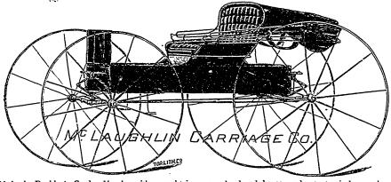
34 wheels, Double A. Grade; 34 axles with wrought iron case hardened boxes, and patent noiseless washers. Body, 20 or 22 in, wide. Top and back removable. Seat full lined, velvet carpet, etc. Special all through.
