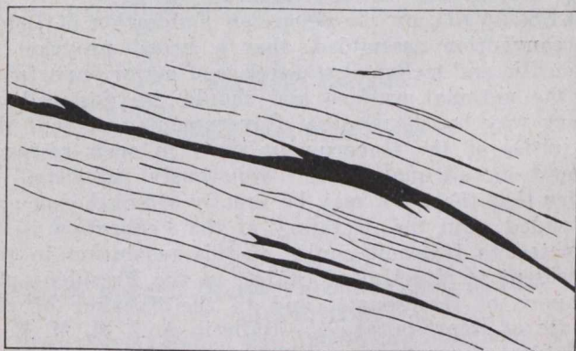
Sketch showing quartz veins at Howey-Cochénour-Willans gold prospect, Holloway township; east walls at depth of 35 feet in shaft. The length of vein system in sketch is about six feet. The main quartz vein is shown by the heavy black part; parallel stringers of quartz occur on each side of the main vein.—Bureau of Mines.
