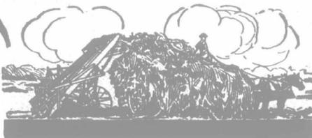
leaves because the self-expanding throat allows hay to pass freely onto wagon without wadding, tangling or jamming. An apron at top keeps hay from spilling or blowing off side of load. Wheels set underneath so it can be taken through gates and operated close to fences, can be coupled on without crawling under wagon, uncoupled without getting off load.
