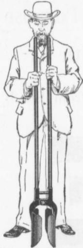
The pick and shovel combined in one, and equally good with loose soil, clay or gravel.
