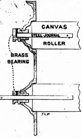
Our outside oiling safety capped end Canvas Rollers. See how the end of the roller is protected. No possibility for damp
