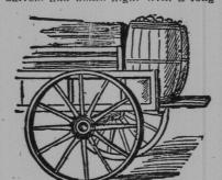
PLATFORM FOR MARKET WAGON. bodled wagon very little climbing is necessary; with a short-bodied wagon constant climbing becomes tiresome The plan herewith shows a board of the wagon and on it barrels, box securely by a rope.-B. D. Thompson,
