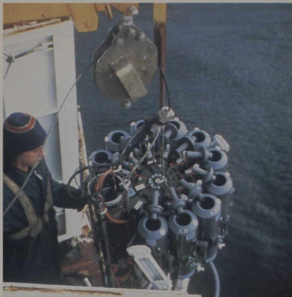
An instrument cluster used for water sampling.
