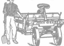
Easy to Load Because the beater is mounted on the rear axle, it is only "hip-high" to the top of the box. Each forkful of manure is put just where it is needed. You can always see into the spreader.
