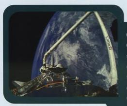
On a NASA space shuttle mission In May 1996, Canadian astronaut Marc Garneau retrieved a satellite in flight Nice Catch! using the Canadarm. He did it with the help of the Space Vision System, a technology developed by NRC that helps astronauts guide the Canadarm with pinpoint accuracy.
